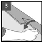
When folding down it is important to start from the corner closest to the previous row, folding down towards the center, and continue towards the opposite long side. During the fold down, make sure the panels are close to each other.
