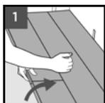
Separate the whole row by carefully lifting up and release the whole row. Fold up the row and release the whole long side.
