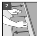
Disassemble the panels by sliding the short ends horizontally. **Never fold up a panel, as this damage the profile.**
