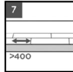
Staggered joint distance i.e. minimum distance between short ends of panels in parallel rows shall not be less than the given length.
