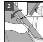
Remove the vertical locking part of the strip with a chisel, put applicable glue on the strip and push the panels horizontally together. Place some spacers between last board and the wall.
